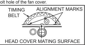
Align the alignment marks on the cam pulley so that they are in line with the head cover mating surface. Be careful ta avoid turning the crankshaft when installing.
