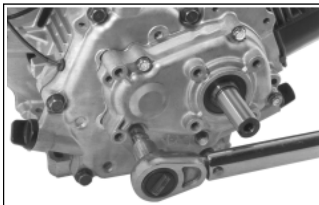
Figure 11-36. CS4, CS6. Torquing Cover Mounting Screws.
