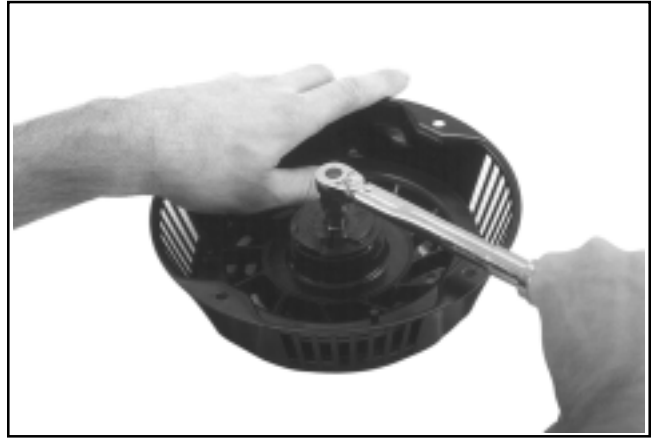
Figure 7-11. Torque Center Mounting Screw.
