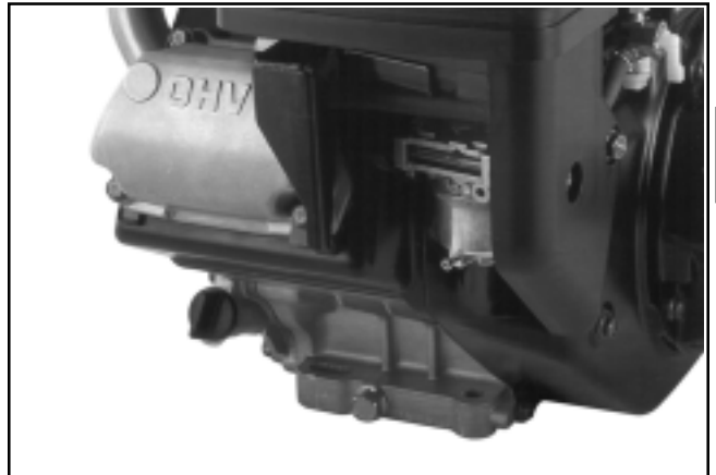
Figure 6-7. CS8.5-12 Left Oil Fill/Level Plug Location.
