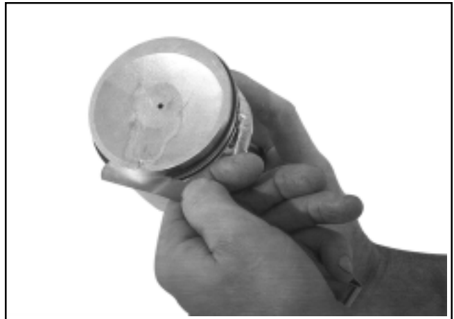
Figure 10-15. Measuring Piston Ring Side Clearance.
