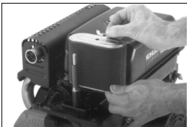
Figure 4-5. Standard Element/Precleaner Assembly.
