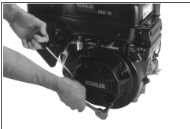
Figure 7-3. Engage Pawls and Tighten Mounting Screws.
