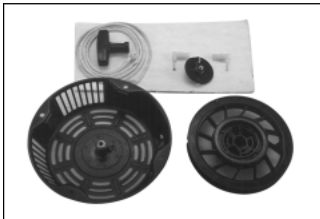
Figure 7-9. Disassembled Retractable Starter.
