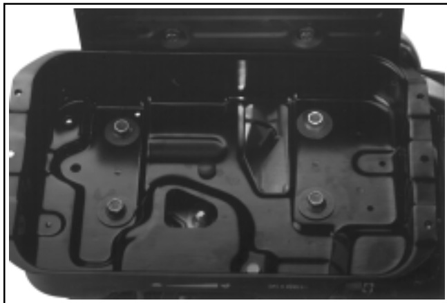
Figure 9-11. CS8.5 (spec. 95xxxx) Fuel Tank Support.
