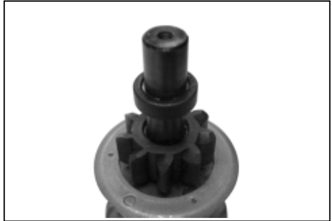
Figure 8-51. Lock Collar around Retaining Ring.
