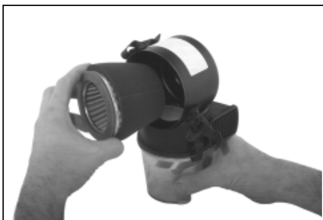
Figure 4-6. Heavy-Duty Element/Precleaner Assembly.
