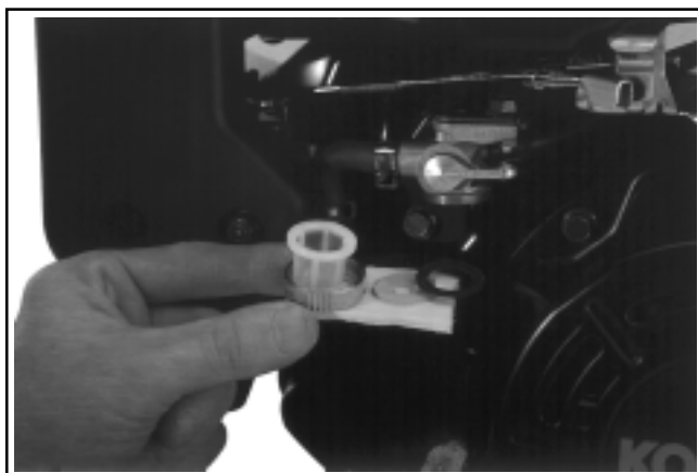
Figure 11-113. CS8.5 (spec. 95xxxx). Shut-Off Valve Details.
