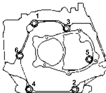
Figure 11-22. CS4, CS6. Closure Plate Torque Sequence.
