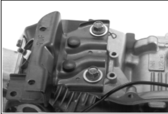
Figure 9-34. CS4, CS6 Left Side Tank Mounting Bracket Details.
