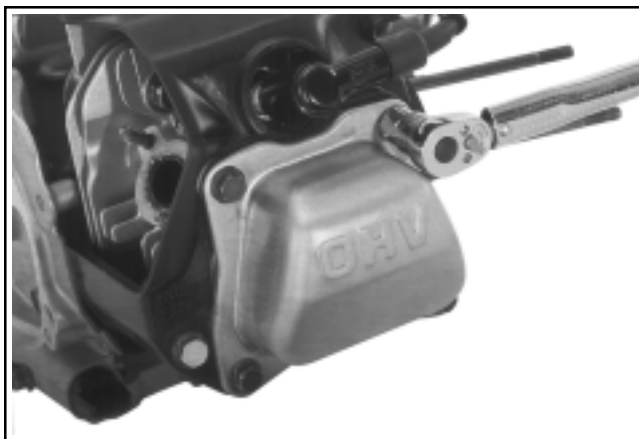
Figure 11-78. CS4, CS6, CS8.5 (spec. 95xxxx). Torquing Valve Cover Screws.
