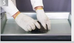
Clean the air cleaner element in warm soapy water, rinse, and allow to dry throughly.
