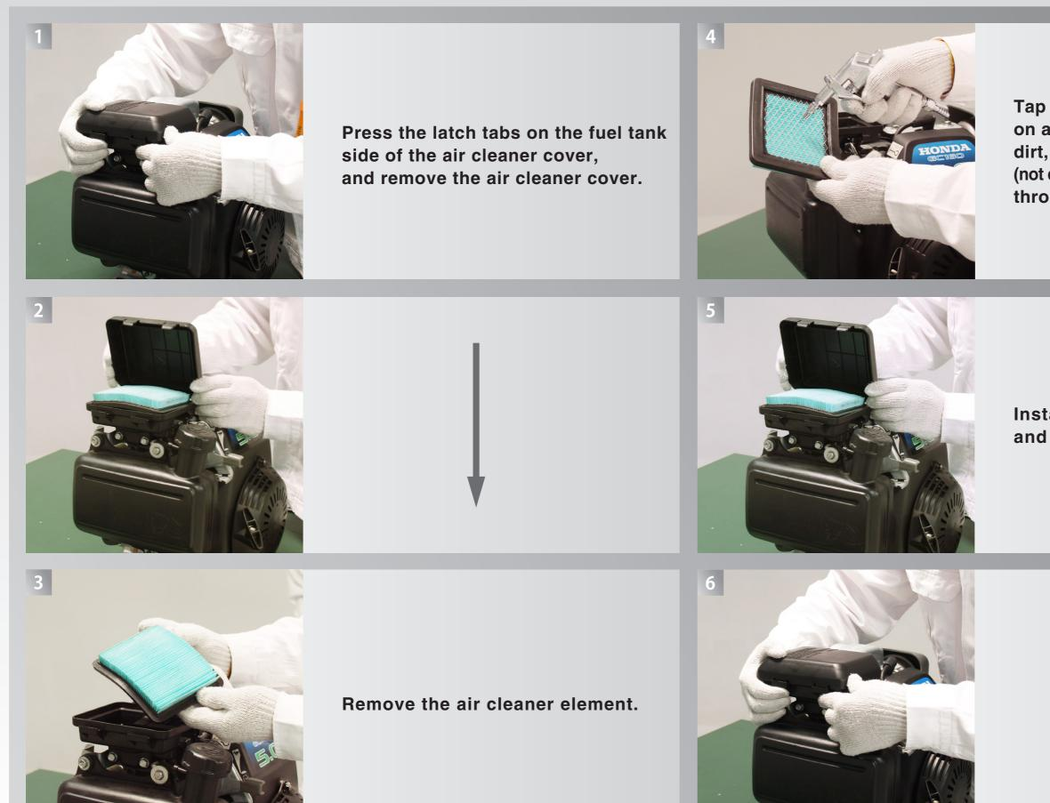
Tap the element lightly several times on a hard surface to remove excess dirt, or blow compressed air (not exceeding 30 psi (207kPa <2.1kgf/cm3) through the filter from the inside out.
